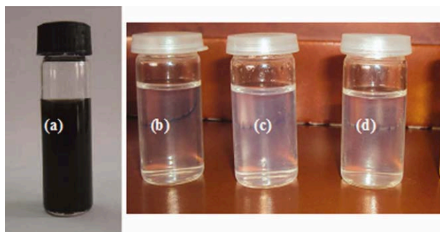
Figure 6 Photos of (a) \text{Fe}_3\text{O}_4 , (b) \text{Fe}_3\text{O}_4 -PAMPS-Na, (c) \text{Fe}_3\text{O}_4 -AM/AMPS1, (d) \text{Fe}_3\text{O}_4 -AM/AMPS3 solutions. [Color figure can be viewed in the online issue, which is available at wileyonlinelibrary.com .]
